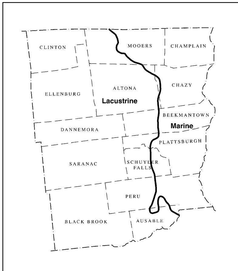
Figure 2.—The Champlain Valley was once inundated by a large glacial Lake Vermont and a subsequent Champlain Sea. The approximate interface between marine deposits (right of the boundary) and lacustrine deposits (left of the boundary) is shown here (Denny, 1974).
